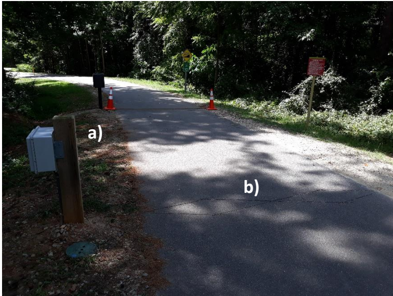
Figure 4. Eco-Counter MULTI with (a) Passive Infrared PYRO in a Wooden Post and (b) Inductive Loop ZELT
