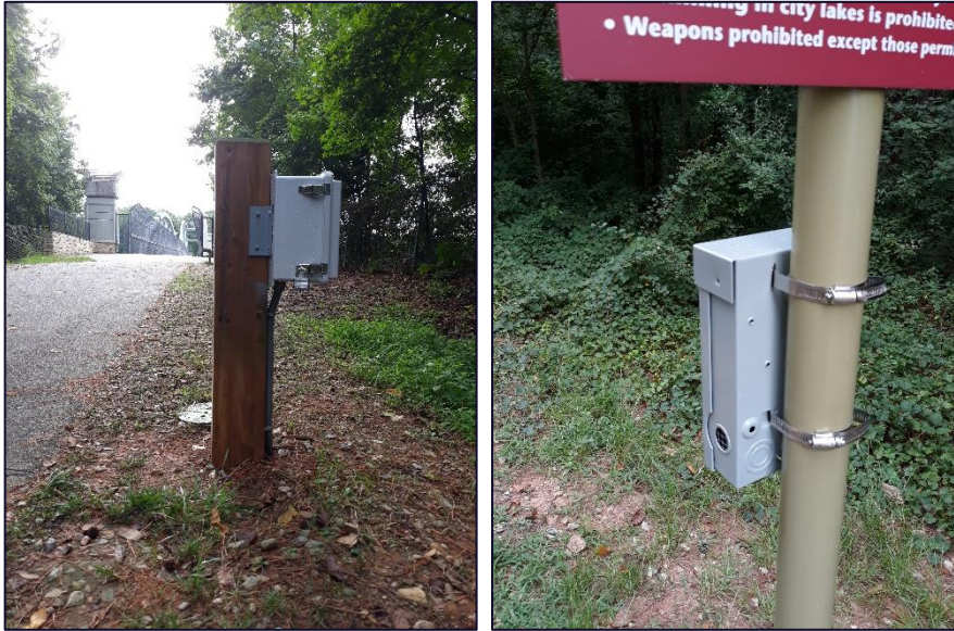
Figure 2. Eco-Counter MULTI with Passive Infrared PYRO in a Wooden Post (left) and TRAFx Trail Counter (right)
